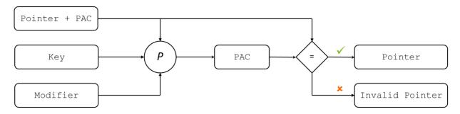
The authentication operation regenerates the PAC and compares it with the value that is stored in the pointer. If authentication succeeds, a pointer without the PAC is returned. If authentication fails, an invalid pointer is returned. This means that an exception is raised if the pointer is used.
