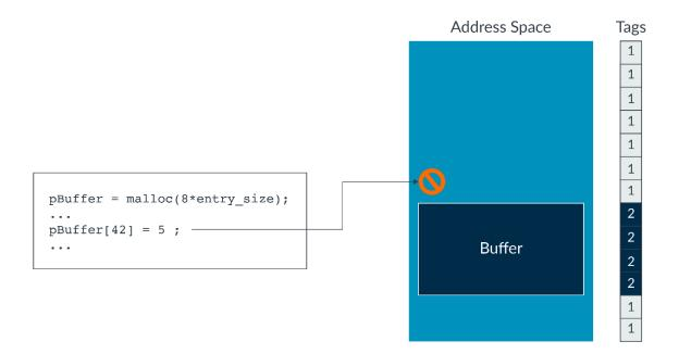
On the call to malloc() the C library will allocate the memory and assign a tag for the buffer. The returned pointer will include the allocated tag. If software using the pointer goes beyond the limits of the buffer, the tag comparison check will fail. This failure will allow us to detect the overrun.
