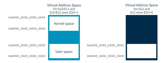
You can see that there are potentially two 2<sup>52</sup> byte address ranges, one at the top of the address space, and one at the bottom of the address space:
