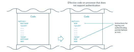
Note: To provide backwards compatibility, this program uses separate instructions to authenticate the LR and return. Ideally the combined authenticate and return instructions, RETAx, would be used. However, the RETAx instruction does not use the NOP instruction space. This means that it is not compatible with a processor that does not support authentication.
