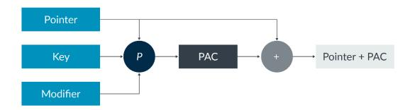
The architecture allows different implementations, for example from different vendors, to use different encryption algorithms. The recommended algorithm is QARMA, which is required by SBSA level 5. ID\_AA64ISAR1\_EL1 reports which algorithm is supported on a specific processor.
