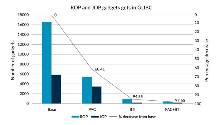
By enabling both pointer authentication and branch target identification, the number of gadgets that are available reduces by 97.65%.
