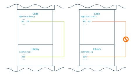
The use of landing pads significantly reduces the number of possible targets for an indirect branch and makes it harder to string chains of gadgets together to form a new program.
