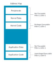
Note: By convention, kernel space is at the top of memory and user space is at the bottom of memory. Although this is not required by the architecture, it is the most common layout and the examples in this guide will follow this convention.
