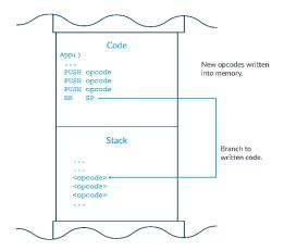
Typically, the memory that is used to launch the attack is stack memory. This is where the name stack smashing comes from. To protect against stack smashing, modern processor architectures, like the Arm architecture, have execution permissions. In Armv8-A, the main controls are execution permission bits in the translation tables. If we focus only on ELO and EL1:
