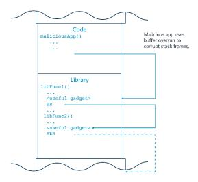
The attacker exploits the fact that BLR or BR instructions can target any executable address, and not just the addresses that are entry points defined by the compiler or developer. This means that the instructions can be hijacked to string gadgets together.
