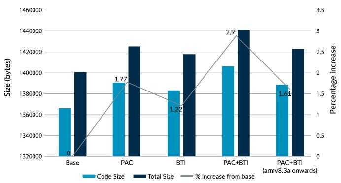
The graph shows that the code size effect on GLIBC is minimal. Even though turning on both the mitigations leads to a 2.9% code size increase, this increase is smaller when compiling with -march=armv8.3-a. Compiling for Armv8.3-A allows the compiler to use fused authenticate and return instructions. This means that, for Armv8.3-A, the code size increase is only 1.6%.
