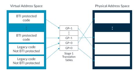
The encoding for BTI instructions, like the pointer-authentication instructions, is allocated within the NOP space. BTI-protected code can still function when run on older processors that do not support BTI, or when GP=0, although without the additional protection.
