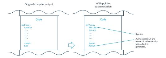
This change makes ROP attacks much harder to launch. This is because, to form the chain of gadgets, the attacker needs to know the location of those gadgets, and correctly signed pointers to those locations. To get a signed pointer it would need access to signing gadget. How is the PAC formed?
